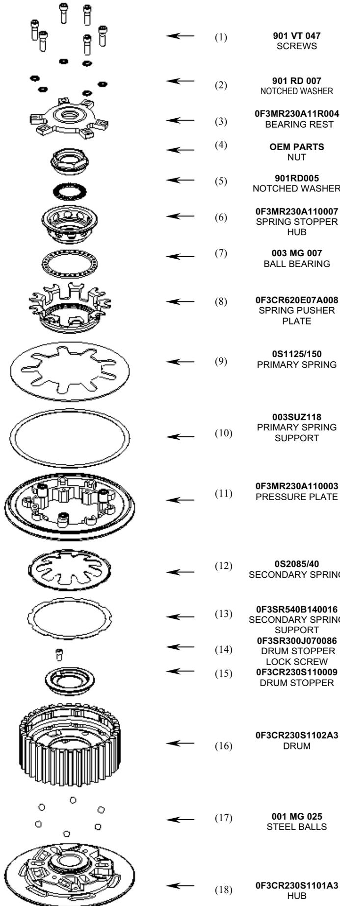
The Drum/Hub group is supplied pre-assembled. **In case of need**, as to check the ramps wear, please see hereinafter the specific procedure to disassemble the Drum/Hub group.
