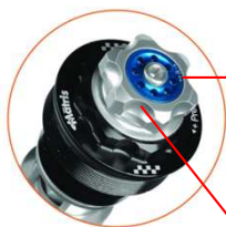
F25SA Sealed cartridge asymmetric system
