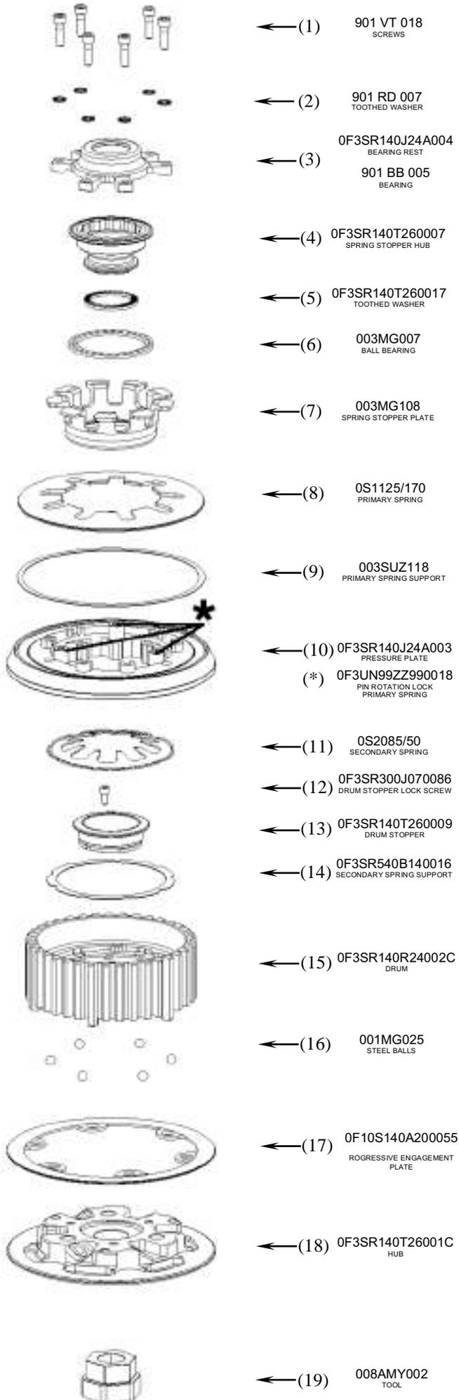
The Drum/Hub group is supplied pre-assembled. **IN CASE OF NEED**, to perform a ramp condition inspection, see below the DRUM/HUB UN-INSTALL PROCEDURE.
