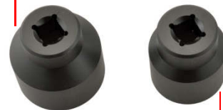
T22 fork cap tool 28 (6 sides)
